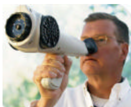
Nasal Ranger made by St. Croix Sensory is a portable odor detecting and measuring device used by Township odor monitors
